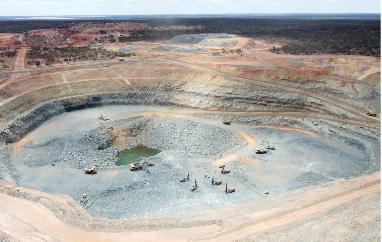
Figure 1 - Missouri open pit mining - sequence changes have optimised operating work area to provide flexibility and improve equipment efficiencies
